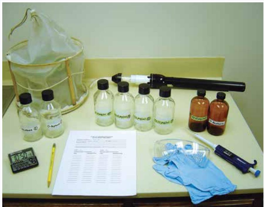
Figure 1: Equipment used for bottle bioassay tests.
